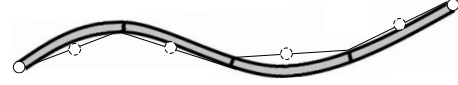
FIG. 13. Incorporating averaged implicit hydrodynamics in the string-of-rods idealization of semiflexible filaments. The string-of-rods idealization considers a semiflexible filament (shown in gray) as a continuously curved string of rods or "segments." The average implicit hydrodynamics is used to solve the hydrodynamic velocities of the end beads (circles with solid outlines), and that of the central representative beads (circles with broken outlines) of the u_1 -projections of the segments. The u_1 -projection of each segment is shown in thin black lines and is along the direction joining the two ends of the segment. Therefore the u_1 -projection of each segment constitutes a section in the implicit hydrodynamics technique. The hydrodynamic drag force due to the hydrodynamic velocities of an end bead enters the string-of-rods formulation as an end force on that segment. The hydrodynamic drag due to the hydrodynamic velocity of a representative bead enters the string-of-rods formulation as the resultant drag force/couple on the u_1 -projection of that segment.
